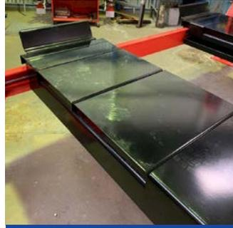
LONG RECESS FOR CUSTOMISED POSITIONING OF TURNTABLE
